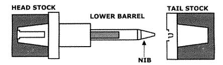
(3) Reverse double ended assembler in head stock. insert twist mechanism in hole provided with brass insert pointing outwards. Now put lower barrel with nib in tail stock. Prise mechanism into indicated line.
